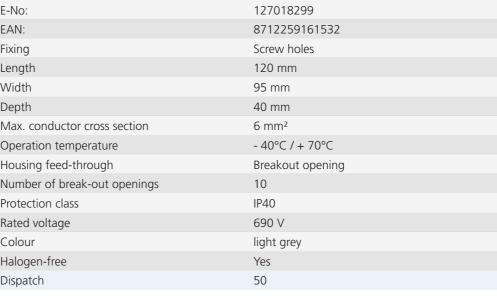
The AK2 modular system can cover a wide range of applications, as it offers the right solution for all installation tasks. The modular system consists of a basic box, a front part and attachment accessories in numerous variants. This allows individually configured boxes to be assembled for pluggable electrical installation.
