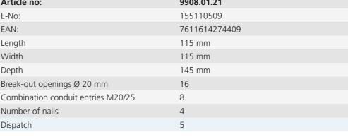
Each flush-mounted junction box has a large number of break-out conduit inlets. They are equally suitable for use with flexible plastic conduits of the corrugated (KRFG) or the smooth (KRF) type. The electrician can easily and quickly insert the conduits into the box or pull them through.
