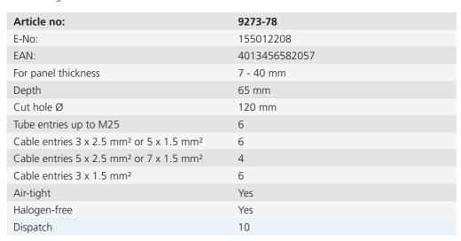
Air-tight  $\emptyset$  120 mm junction box with ECON® technology for an energy-efficient electrical installation in accordance with GEG. Extremely easy fitting thanks to toolless cable and conduit entry. The sealing membranes guarantee permanent air-tightness and at the same time retention of the cable or conduit. The large box volume provides plenty of installation space for various cable connections.
